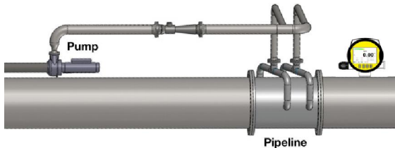
Figure 2. SB-TT as a pipeline temperature measurement
